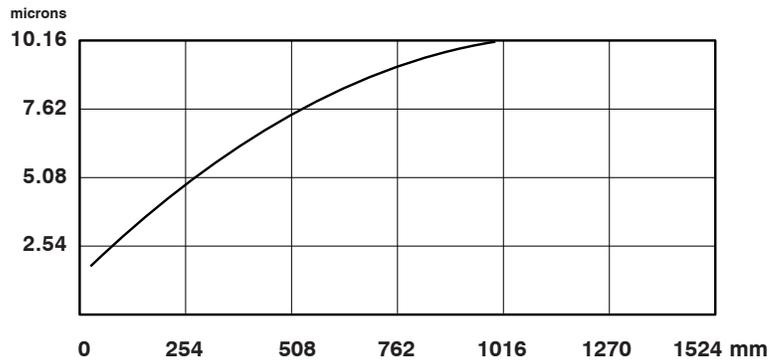
Maximum deviation from parallelism between the vee groove face and datum faces of each way bar is shown in the graph. Actual accuracy achieved depends on proper installation.
