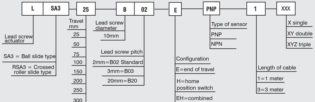
Designed for NEMA 23 motor frame. Supplied with coupling for 8mm motor shaft.
