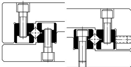
Mounting holes in the way bars are threaded, and also counterbored to alternatively permit using the next smaller size screw with threaded mounting holes in the user's components.
